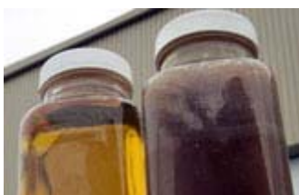
Two sample jars, one showing used restaurant frying grease (R) and the second showing the refined end product of biodiesel, produced at the Rothsay plant in Quebec, Canada. The plant uses recycled restaurant grease as well as old foodstuff to produce biodiesel (Photo: Reuters)
